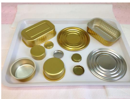
Fig. 11: Samples of cans and caps lacquered with BIOCOPAC varnish.
